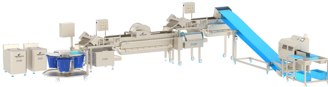
HS-ES in a vegetable processing line for cutting, washing and drying vegetables
